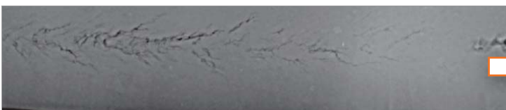
Weld X-ray before Image Enhancement
