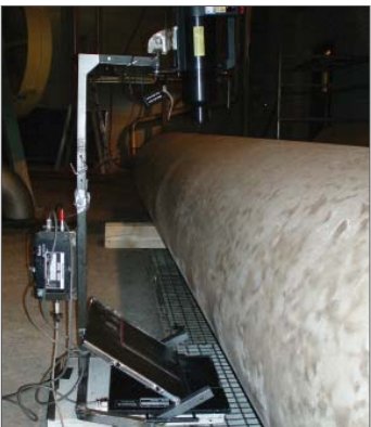
Glass Fibre Profile Inspection
